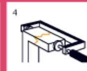
4 Assemble carefully and remove any excess adhesive with a sharp blade once partially set.
