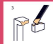
3 Make sure both surfaces are clean and dry. Apply to both surfaces of the joint.
