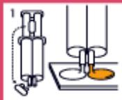
1 Snap off the resealable cap from between the syringe plungers and break off the end seal. Depress the plunger to dispense equal amounts of both components onto a clean disposable surface. Re-fit the cap to close the nozzle.
